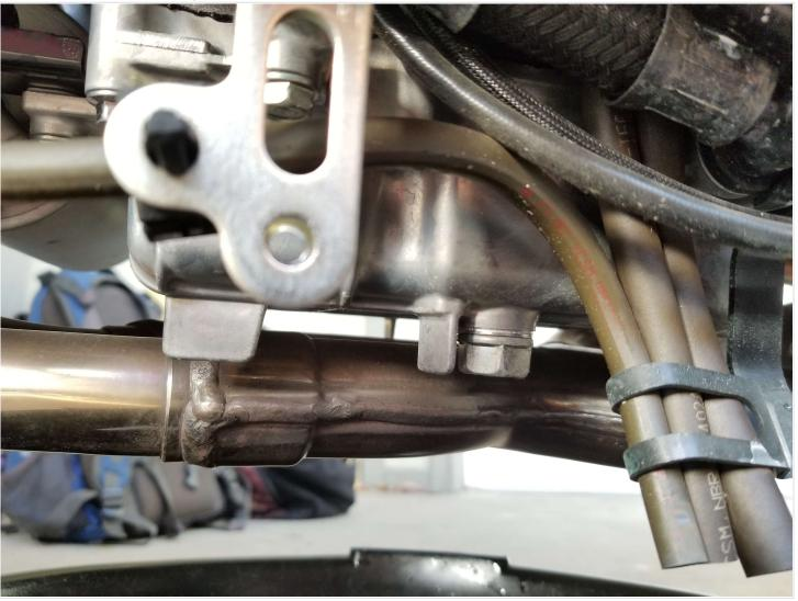
5. Remove 10mm bolt securing lower part of the lower radiator (accessible via left-hand side.)
